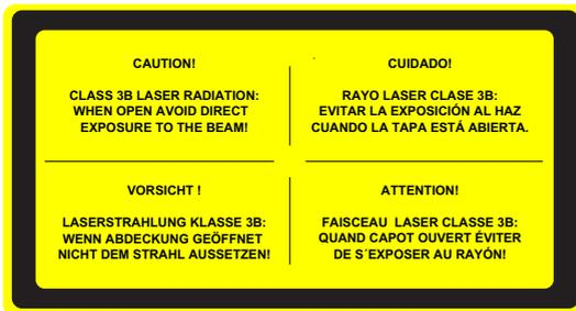
The digitizer is a Class 1 Laser Product. It uses one laser diode of a 80 mW type, classification class IIIb, wavelength 640-670 nm. The laser beam divergence is 120 - 350 mrad. The laser beam's deflection frequency is 70 1/s up to 90 1/s.
