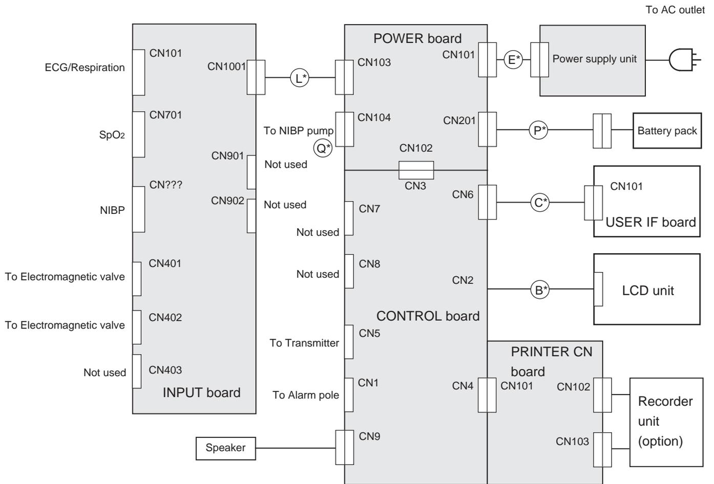
\* About wire harnesses B, C, E, L, P and Q, refer to Section 7 Replaceable Parts List.
