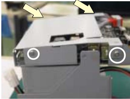
2. Remove the 6 screws which secure the insulation sheet and NIBP socket holder to the INPUT board.
