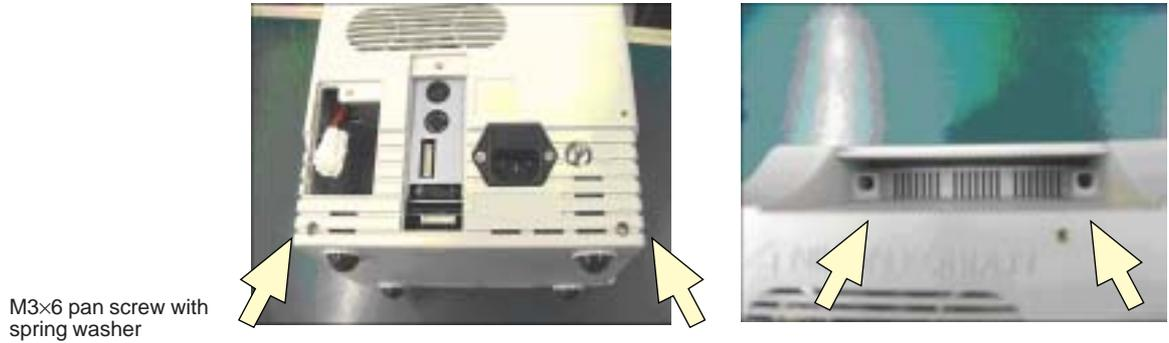
2. Remove the screw which secures the recorder blank panel to the instrument and remove the blank panel.
