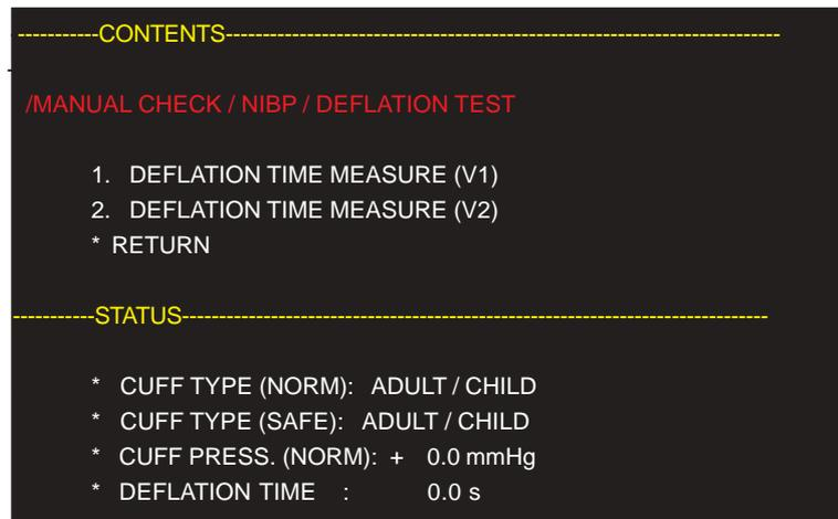
1. DEFLATION TIME MEASURE (V1): Measures the time when the valve 1 is open and the cuff pressure reaches 15 mmHg after 300 mmHg pressure is applied to the 700 cc dummy cuff.
