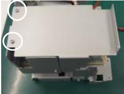
14. Disconnect the 2 wire harnesses from the power supply unit and remove the 4 screws which secure the power supply unit to the chassis block. Remove the power supply unit from the chassis block.
