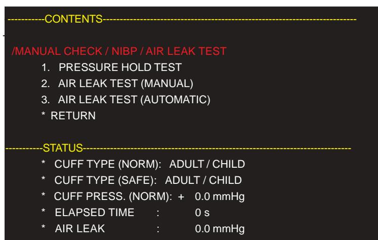
1. **PRESSURE HOLD TEST:** Measures the pressure difference between the two cuff pressures at 10 seconds after and at 20 seconds after 300 mmHg pressure is applied to the 700 cc dummy cuff.
