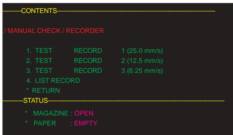
1. TEST RECORD 1: Records a triangle wave at 25.0 mm/sec paper speed. 3 peaks are recorded on the paper. The peak to peak length along the time scale is 25 mm.
