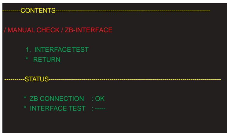
1. INTERFACE TEST: Checks the connection between the instrument and ZB-900P/ZS-900PK transmitter, and checks the communication between the instrument and ZB-900P/ZS-900PK transmitter.
