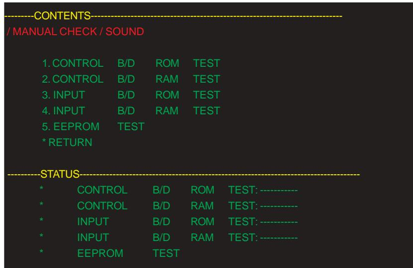
1. CONTROL B/D ROM TEST: Calculates the check sum of the program stored in the ROM on the CONTROL board and compares the calculated sum with a check sum stored in the ROM.
