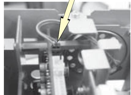
7. Remove the following 3 screws. From the chassis block, remove the POWER board, CONTROL board and PRINTER CN board (including the optional recorder unit if it is built in the instrument). If there is no recorder unit, go to step 10.
