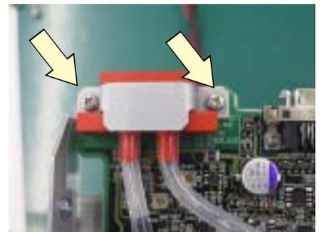
3. Disconnect the air tube from the NIBP pump.
