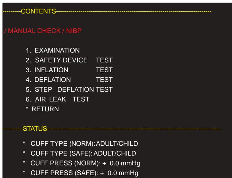
**CUFF TYPE (NORM):** Indicates the type of the air hose connected to the instrument, “ADULT/CHIL” or “NEONATAL”. The air hose type is recognized by the measurement circuit.
