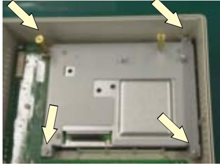
6. Remove the 4 screws which secure the holder to the LCD unit. Remove the holder from the LCD unit.
