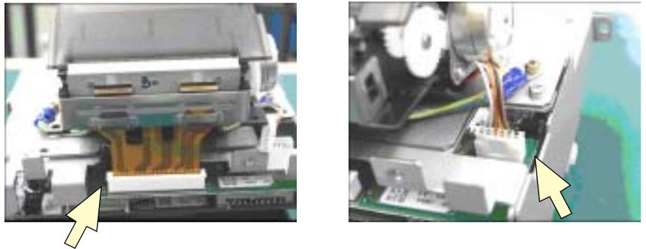
7. Assemble the instrument by reversing steps 1 to 4.
