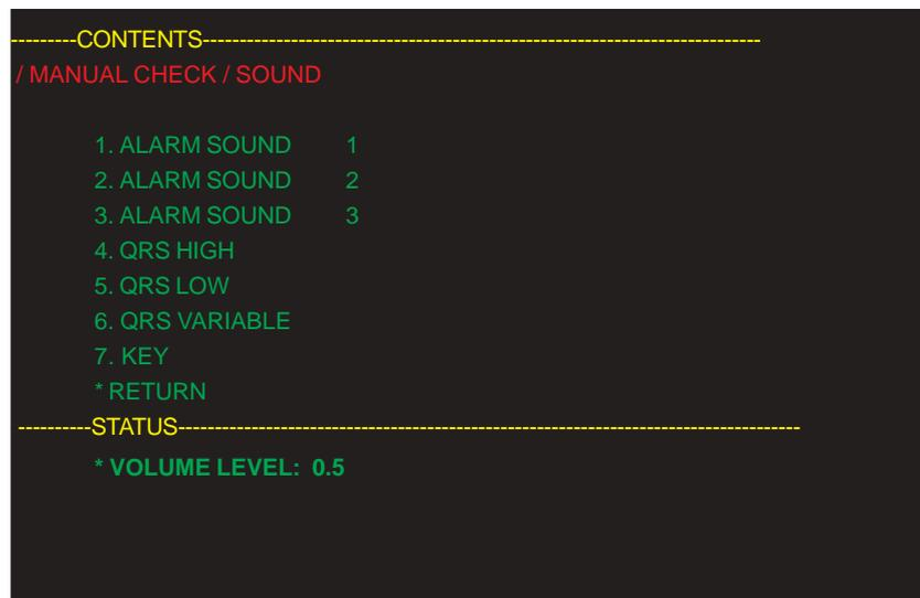
1. ALARM SOUND1: Generates the alarm type 1 (continuous sound) sound.
