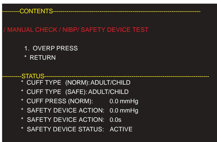
1. OVER PRESS: Checks the safety circuit operation when 300 to 315 mmHg pressure is applied to the 700 cc dummy cuff.
