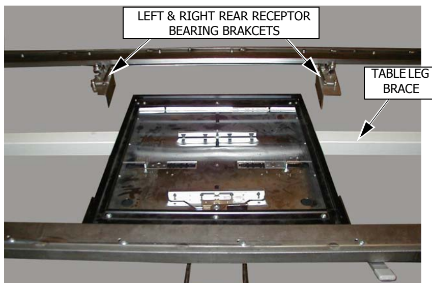
Figure 3-6. Receptor Cabinet Fully Installed
