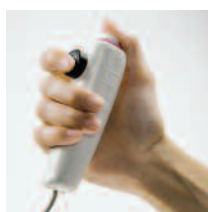
The hand-held switch includes a collimator light to verify image region of interest.
